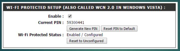
Most wireless routers provide a feature called Wi-Fi Protected Setup (WPS)
