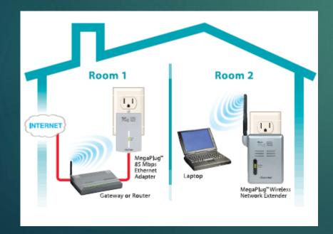
A Powerline connection can also be used to connect an access point to a router outside of range
