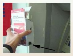
The PIN reading camera being installed on the ATM is housed in an innocent looking leaflet enclosure.
