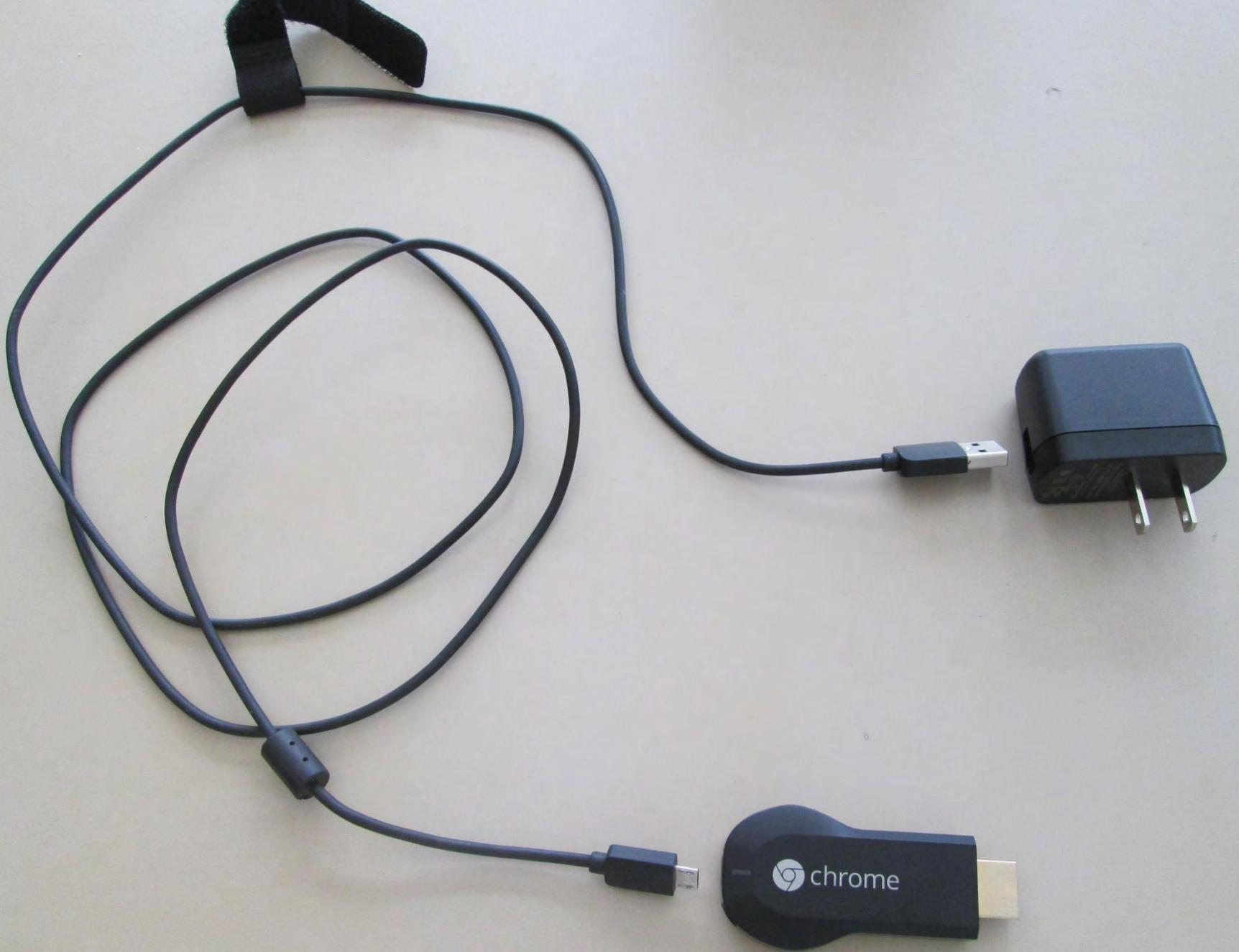
**USB A plug of cable plugs into USB A port of power adapter**
